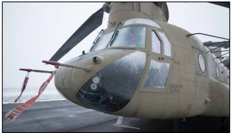
Figure 2. CH-47F with pitot tube covers marked "Remove Before Flight"
