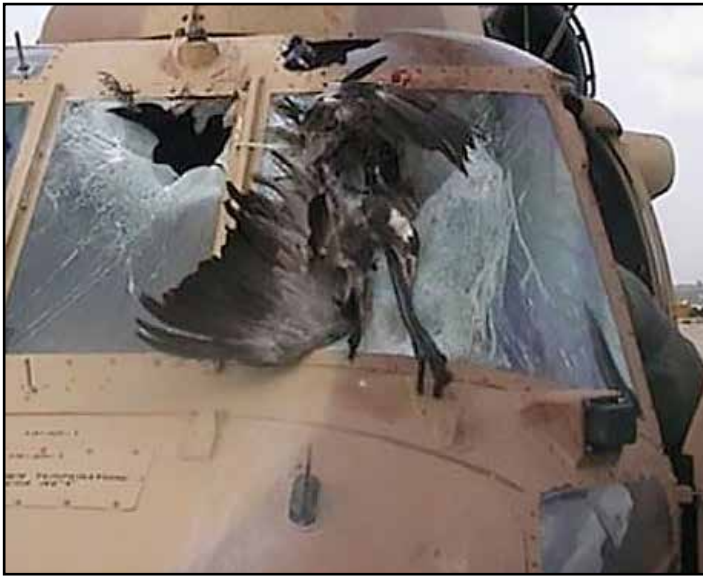
Bird strikes are problems the world over. This photo shows an Israeli Air Force UH-60 Blackhawk after a bird strike. Photo: US Air Combat/Wikimedia Commons
